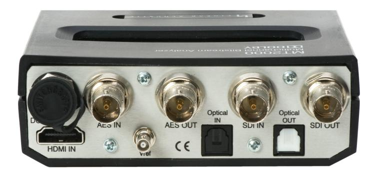
The Linear Acoustic MT2000 Bitstream Analyzer is a portable, handheld diagnostic tool that can monitor and generate Dolby Digital, Dolby Digital Plus, Dolby E, and PCM bitstreams.
