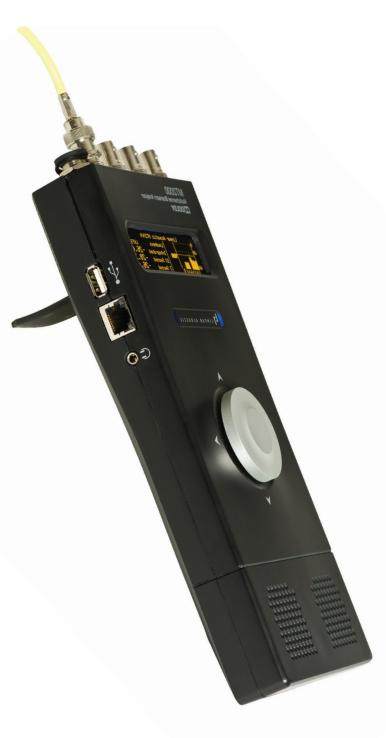
The Linear Acoustic MT2000 accepts signals via AES, TOSLINK™ optical, 3GHz SDI, or HDMI connectors. The unit identifies the format of the selected input signal and activates the appropriate built-in decoder. Monitoring capabilities include error detection at the AES3 layer and within the coded audio layers, including SMPTE 337 formatting information and Dolby E guard band position.
